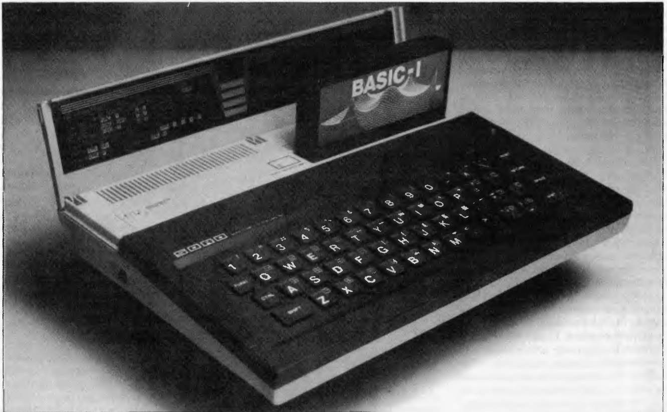
Hinged lid lifts off to allow insertion of cartridges
